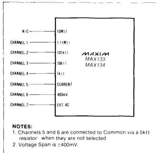
Figure 12. MAX133/134 Input Section used as a Multiplexer.
