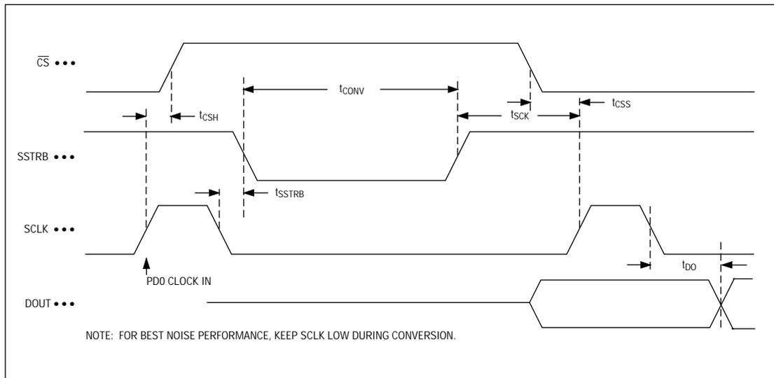
Figure 9. Internal Clock Mode SSTRB Detailed Timing
