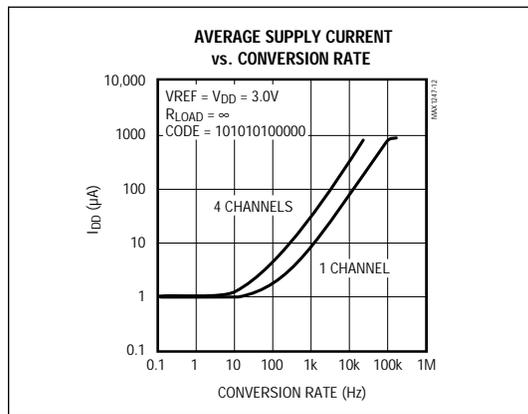
Figure 12. Average Supply Current vs. Conversion Rate
