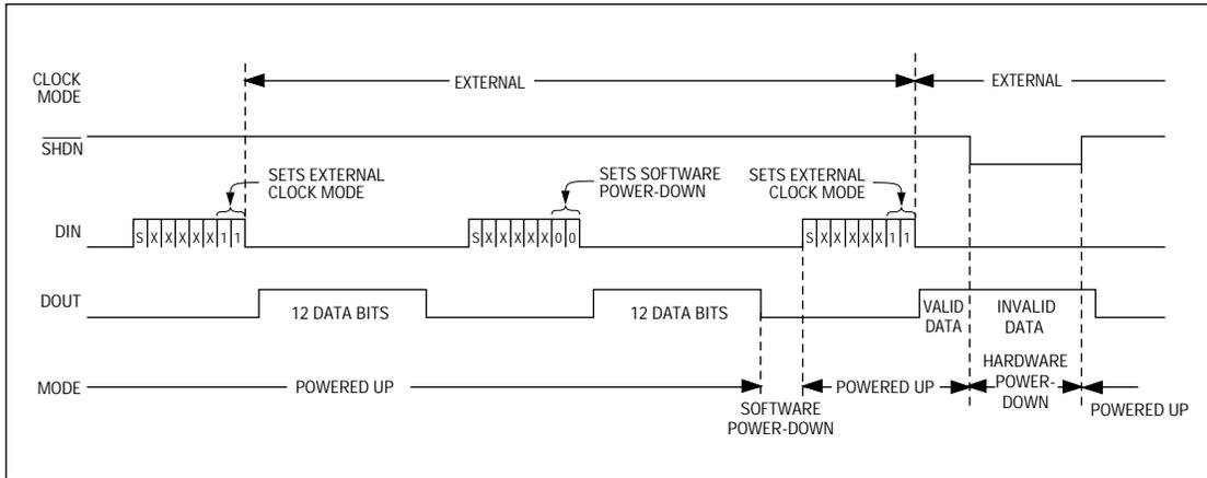
Figure 11a. Timing Diagram Power-Down Modes, External Clock
