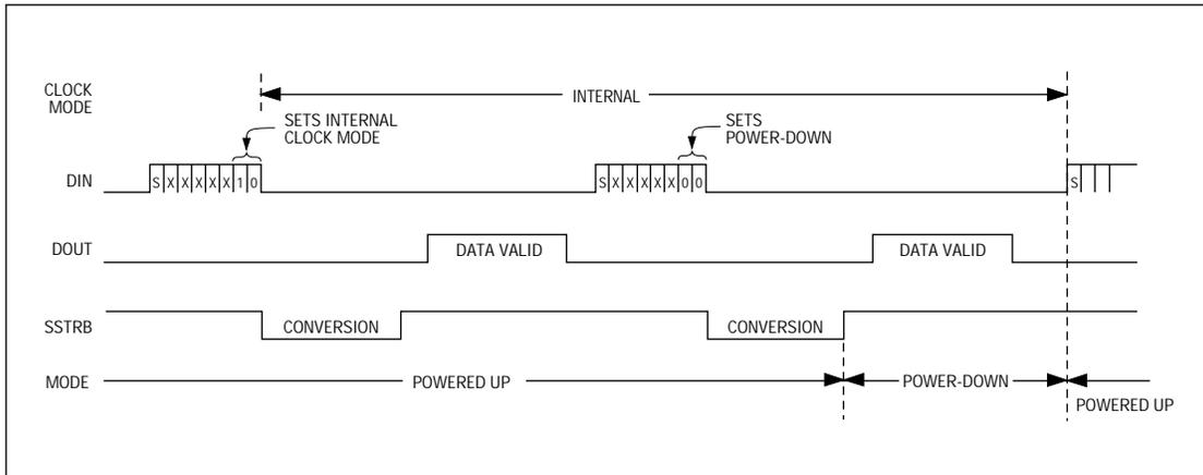
Figure 11b. Timing Diagram Power-Down Modes, Internal Clock
