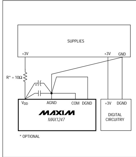
Figure 15. Power-Supply Grounding Connection
