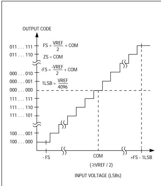
Figure 14. Bipolar Transfer Function, Full Scale (FS) =  $V_{REF} / 2 + COM$ , Zero Scale (ZS) = COM
