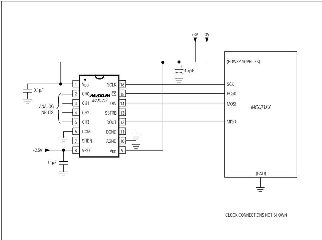
Figure 16. MAX1247 QSPI Connections
