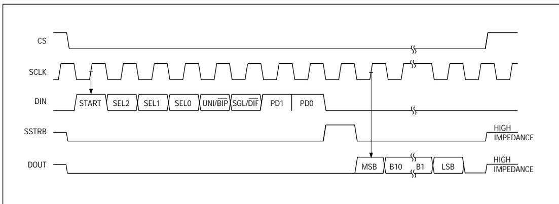
Figure 18. TMS320 Serial-Interface Timing Diagram
