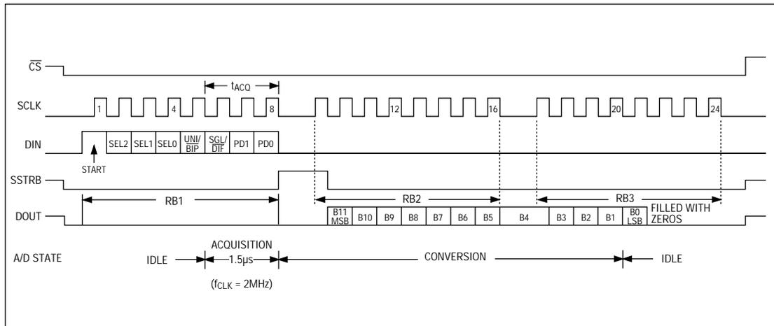
Figure 5. 24-Clock External-Clock-Mode Conversion Timing (Microwire and SPI Compatible, QSPI Compatible with  $f_{CLK} \leq 2\text{MHz}$ )
