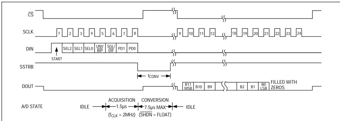
Figure 8. Internal Clock Mode Timing
