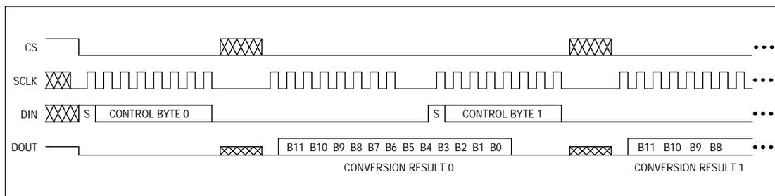
Figure 10b. External Clock Mode, 16 Clocks/Conversion Timing
