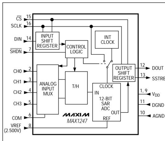
Figure 3. Block Diagram
