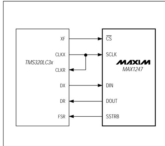
Figure 17. MAX1247-to-TMS320 Serial Interface
