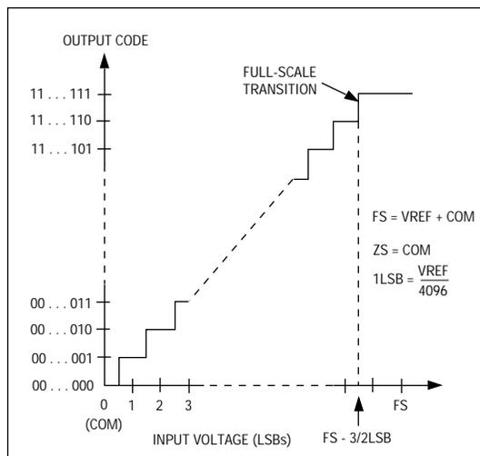
Figure 13. Unipolar Transfer Function, Full Scale (FS) = VREF + COM, Zero Scale (ZS) = COM
