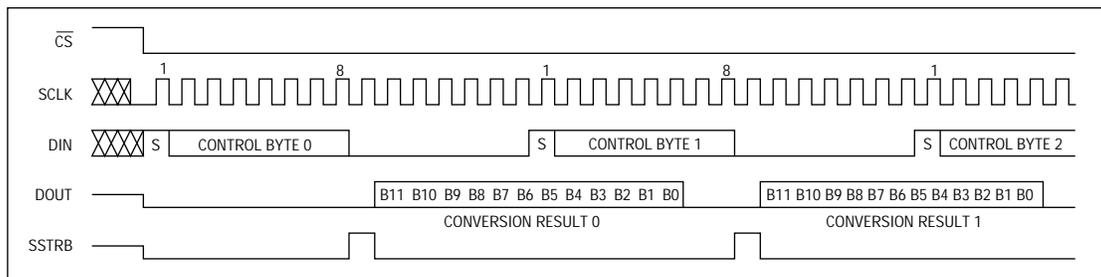
Figure 10a. External Clock Mode, 15 Clocks/Conversion Timing
