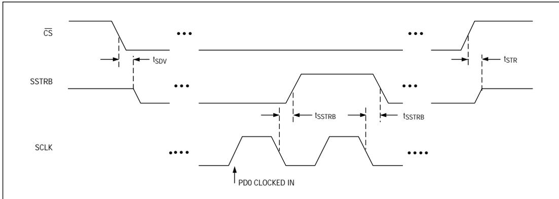
Figure 7. External-Clock-Mode SSTRB Detailed Timing
