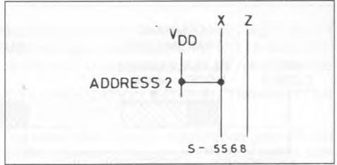
The Address inputs have internal pull-downs which are disabled during stand-by.
