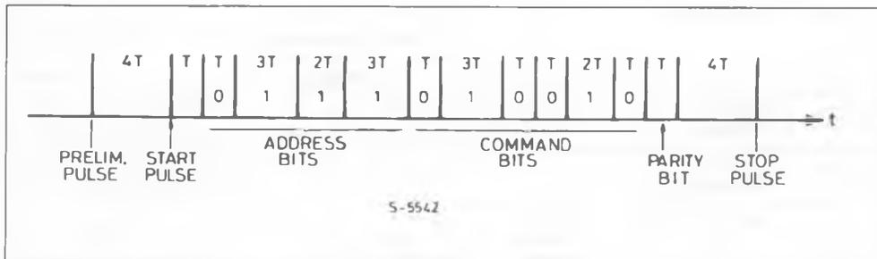
sequently, a word in which the binary digit 0 occurs ten times has a total duration of  $21T$ . A word containing ten "1s" has a duration of  $36T$ . (see Example)
