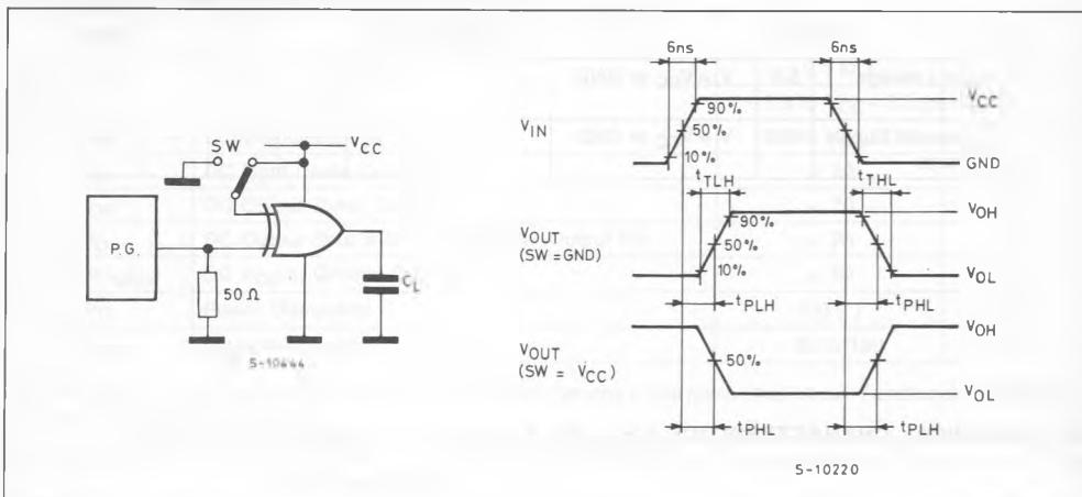
TEST CIRCUIT  $I_{CC}$  (Opr.)
