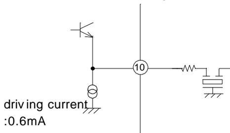
In the split system, the carrier signal to SIF provided from pin 10 through an emitter follower. And, please open this pin, when it is used INTER.
