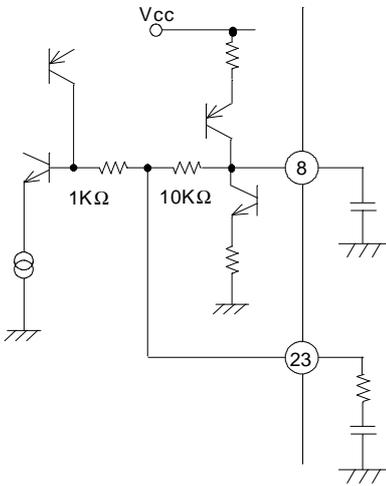
2-pin filter characteristics are available by utilizing the dynamic AGC circuit. And AGC speed can be changed, if pin-23 on the external resistors is variable.
