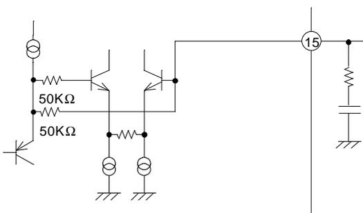
Frequency characteristic of audio output is decided with 15-pin external capacitor value. And audio output amplitude can make it small when it connected 15-pin external capacitor and resistance in series.
