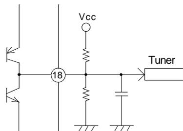
Since an AFT output is provided by a high impedance source, the detection sensitivity can be set by an external resistor.
