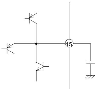
AGC speed can be changed by this pin's external capacity.
