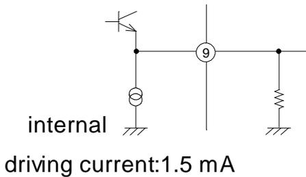
An output amplitude is positive 0.6Vp-p in case of 87.5% video modulation.
