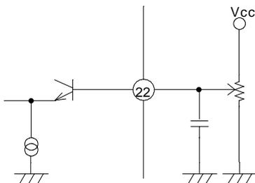
An applied voltage to the pin 22 is for changing a RF AGC delay point.
