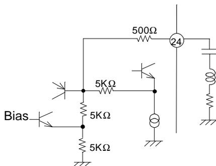
Both the external coil and capacitor determine the frequency response of EQ output.
