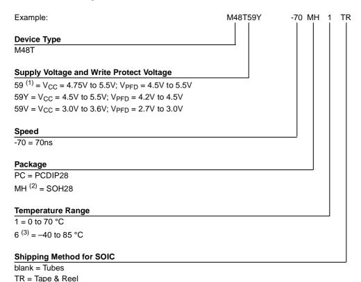
Note: 1. The M48T59 part is offered with the PCDIP28 (i.e. CAPHAT) package only.
