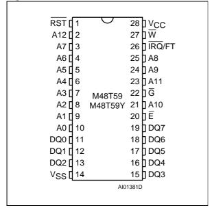
Figure 2B. SOIC Connections
