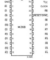
CS1 enables the outputs 01 to 08 CS2 enables the outputs 09 to 12
