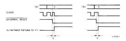
In both the cases the delay  $\tau$  (in the outputs without return to "1") is defined through the constant R1 C1  $\geqslant$  10  $\mu$ sec.
