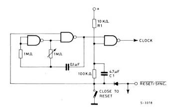
Ext. Reset/Sync. is a bidirectional pin. Used as an input it can reset the circuit as shown in the timing diagram and used as an output it can drive the reset of other devices.
