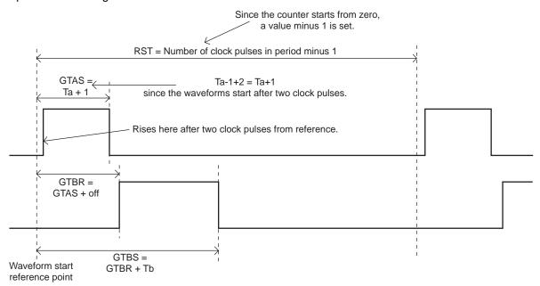
The drive waveforms are set using four parameters: RST, GTAS, GTBR and GTBS.
