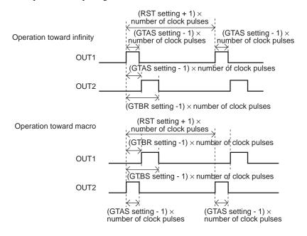
Sequence of initial setting operation ("on" or "off" can be set by the serial settings.) When M/I register =  $00 \rightarrow$  Movement toward infinity position
