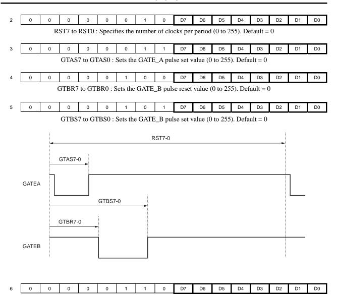
STP7 to STP0 : Specifies the number of output pulse steps with regard to DRIVE input (1 to 256). Default = 1 The setting value range is handled as the data value plus 1.
