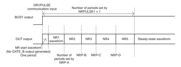
For example, when NRPULSE1 is set to 15, NRP-A to 3, NRP-B to 6, NRP-C to 9, and NRP-D to 12, one period of the NR start waveform (no GATE\_B output) is output, followed by three periods of the NR1 waveform, three periods of the NR2 waveform, three periods of the NR3 waveform, three periods of the NR5 waveform, and then STP x DRVPULSE periods of the steady-state waveform.
