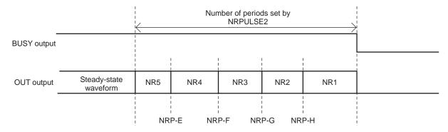
The fall waveforms are output in order from the NR5 waveform to the NR1 waveform. The switching timing is set in the same manner as that for rise operation.
