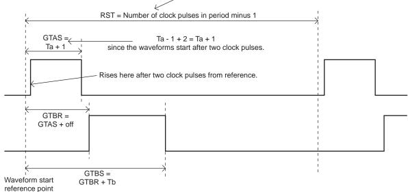
The drive waveforms are set using four parameters: RST, GTAS, GTBR and GTBS.
