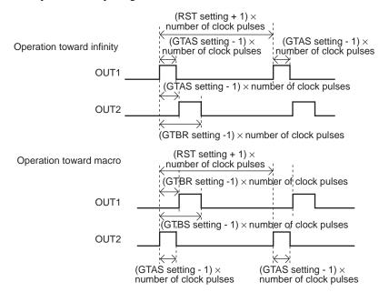
Sequence of initial setting operation ("on" or "off" can be set by the  $I^2C$  settings.) When M/I register =  $00 \rightarrow$  Movement toward infinity position
