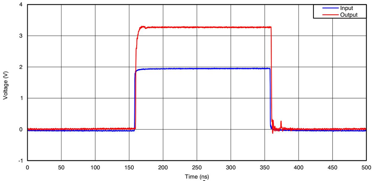
**Figure 8. Captured Waveform From Above I<sup>2</sup>C Set-Up (1.8 V to 3.3 V at 2.5 MHz)**
