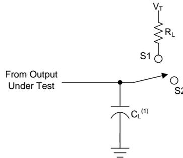
(1)  $C_L$  includes probe and jig capacitance.
