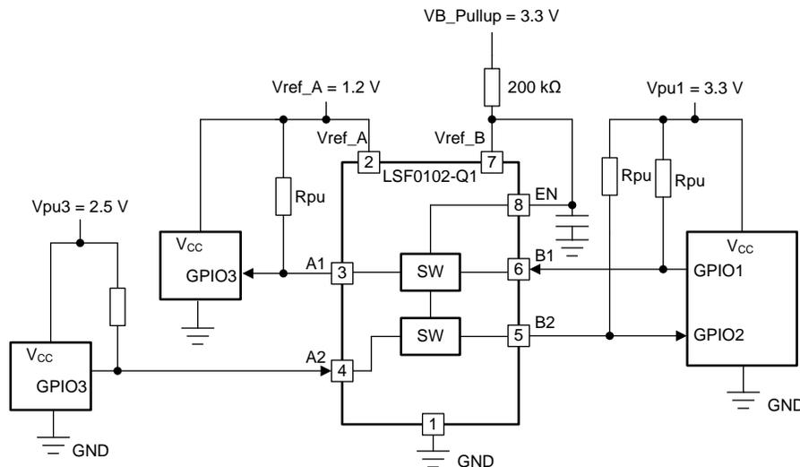
Figure 7. Bidirectional Translation to Multiple Voltage Levels
