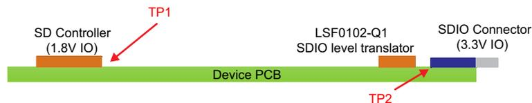
**Figure 10. Device Placement**
