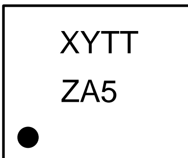
Figure 4. Top View 25 – Bump micro SMD Marking X = Plant Code Y = Date Code TT = Die Traceability ZA5 = LMV1099TL
