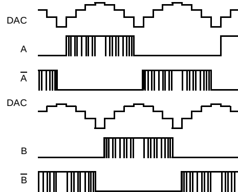
Figure 11: Stepper Motor Waveform - LM9831 Signals
