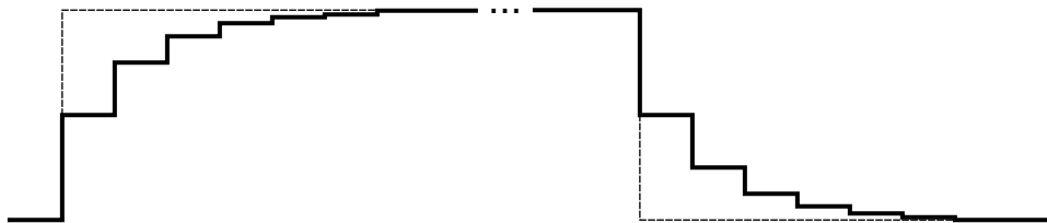
Figure 22. AVS Reference Voltage Large Step With Slew Rate Control (Solid Line) And Without Slew Rate Control (Dash Line)
