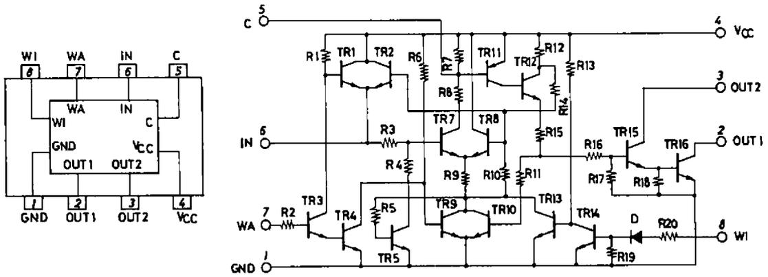
Sample Application Circuit : Asynchronous intermittent wiper control
