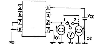
Test Circuit 2 :  $V_{OL1}, V_{OL2}, SW_1, SW_2$
