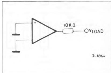
Figure 4 : Fault Current Test Circuit.
