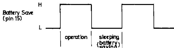
The battery-save function extends battery life for intermittent device operation. The LA8610M is operational when pin 15, the battery-save control pin, is High ( $V_{CC} \pm 0.6\text{V}$ ). When pin 15 is Low, the internal circuits are disabled to reduce power consumption.
