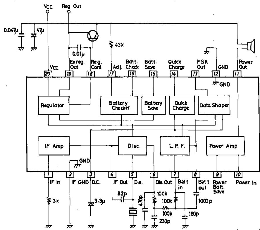
Unit (resistance:  $\Omega$ , capacitance: F)
