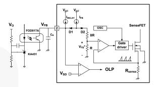
Figure 16. Pulse Width Modulation (PWM) Circuit
