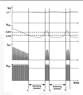
Figure 21. Burst-Mode Operation
