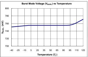
Figure 8. Burst-Mode Voltage (V<sub>BURH</sub>) vs. Temperature
