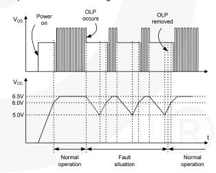
**Figure 17. Auto Restart Protection Waveforms**
