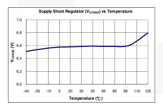
Figure 14. Supply Shunt Regulator (V<sub>CCREG</sub>) vs. Temperature
