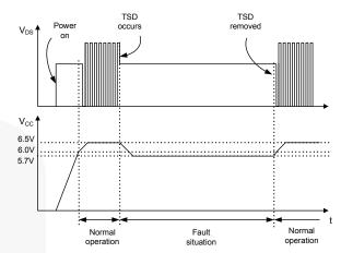
Figure 19. Over-Temperature Protection (OTP)
