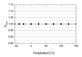
Figure 9. Maximum Duty Cycle (D<sub>MAX</sub>) vs. T<sub>A</sub>
