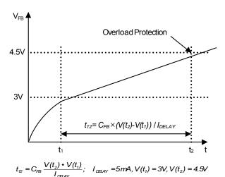
Figure 18. Overload Protection (OLP)
