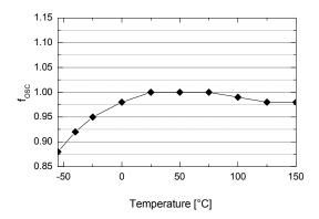
Figure 8. Operating Frequency (fosc) vs. T<sub>A</sub>
