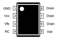
Figure 3. Pin Configuration (Top View)
