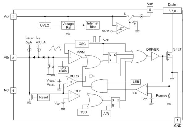
Figure 2. Functional Block Diagram of FSQ211
