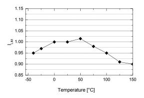
Figure 10. Peak Current Limit (I<sub>LIM</sub>) vs. T<sub>A</sub>
