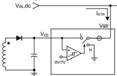
Figure 14. Internal Start-up Circuit
