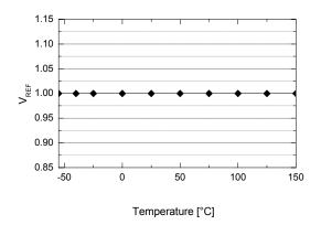
Figure 4. Reference Voltage (V<sub>REF</sub>) vs. T<sub>A</sub>
