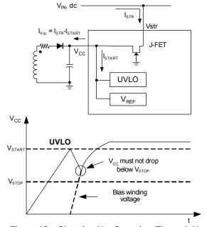
Figure 15. Charging V<sub>CC</sub> Capacitor Through Vstr
