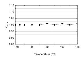
Figure 7. Stop Threshold Voltage (V<sub>STOP</sub>) vs. T<sub>A</sub>
