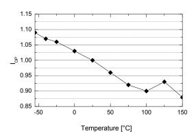
Figure 5. Operating Supply Current (I<sub>OP</sub>) vs. T<sub>A</sub>
