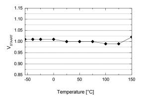
Figure 6. Start Threshold Voltage (V<sub>START</sub>) vs. T<sub>A</sub>
