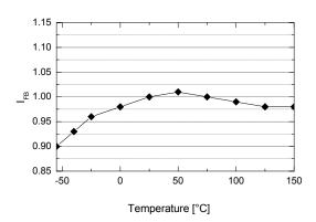
Figure 11. Feedback Source Current (IFB) vs. TA
