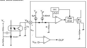
Figure 16. PWM and Feedback Circuit
