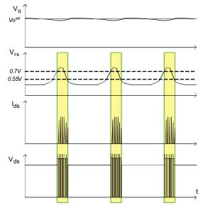
Figure 21. Burst Operation Function
