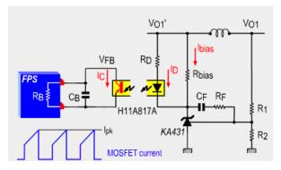
Figure 23. Typical Feedback Network of FPS™
