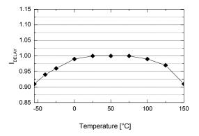
Figure 12. Shutdown Delay Current ( $I_{DELAY}$ ) vs.  $T_A$
