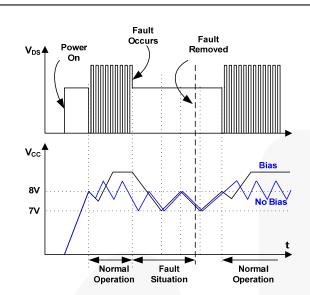
Figure 18. Auto-Restart Protection Waveforms
