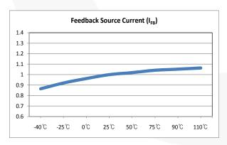
Figure 8. Feedback Source Current vs. Temperature
