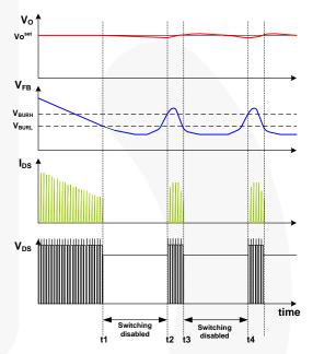
Figure 23. Burst-Mode Operation
