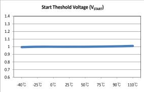
Figure 6. Start Threshold Voltage vs. Temperature
