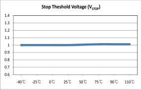
Figure 7. Stop Threshold Voltage vs. Temperature
