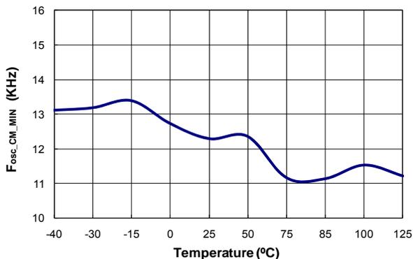
**Figure 13. Minimum Frequency at CCM (f<sub>OSC-CM-MIN</sub>) vs. Temperature**
