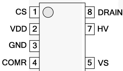
Figure 5. Pin Configuration
