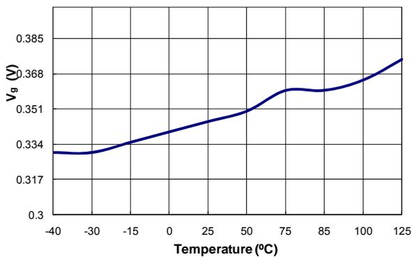
**Figure 17. Green Mode Ending Voltage on EA\_V (V<sub>G</sub>) vs. Temperature**
