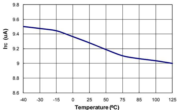
Figure 18. IC Bias Current ( $I_{bc}$ ) vs. Temperature
