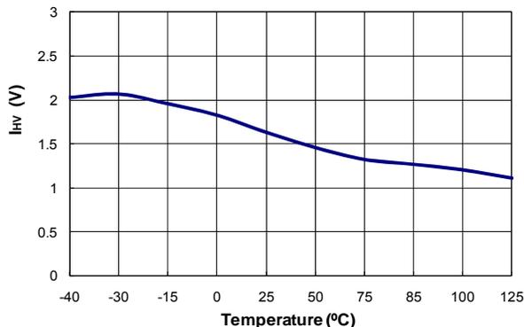
**Figure 14. Supply Current Drawn from HV Pin (I<sub>HV</sub>) vs. Temperature**
