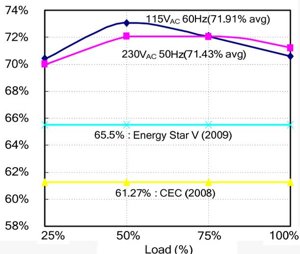
Figure 30. Measured Efficiency
