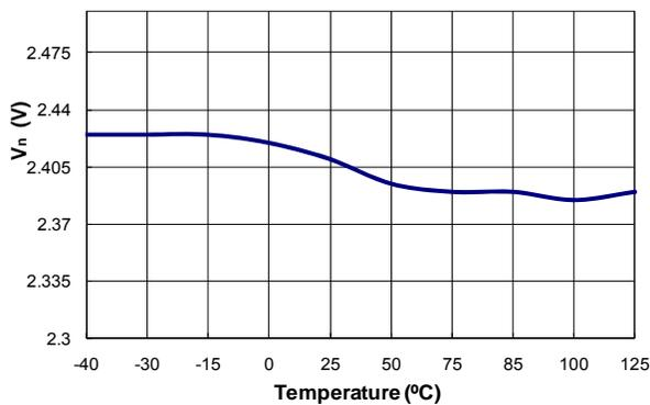
**Figure 16. Green Mode Starting Voltage on EA\_V (V<sub>N</sub>) vs. Temperature**
