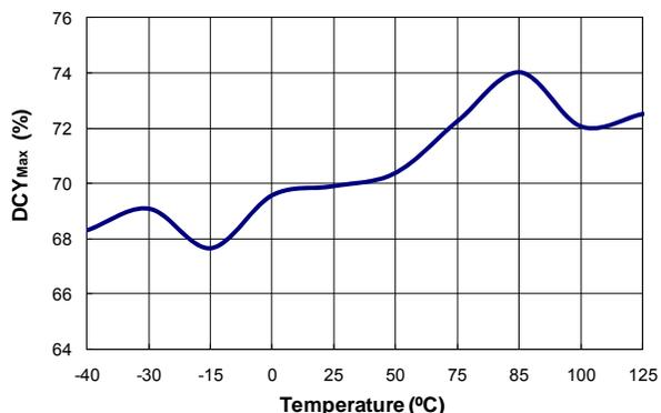
Figure 23. Maximum Duty Cycle ( $DCY_{MAX}$ ) vs. Temperature
