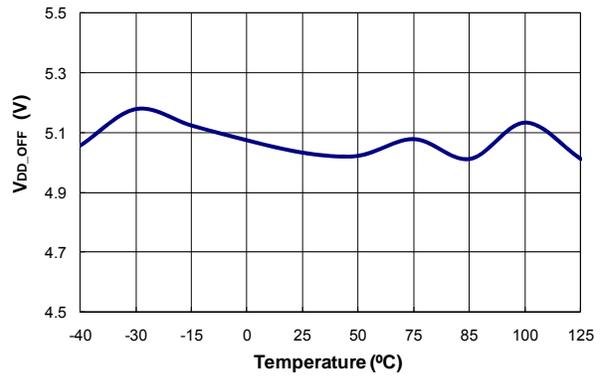
**Figure 7. Turn-Off Threshold Voltage ( $V_{DD-OFF}$ ) vs. Temperature**
