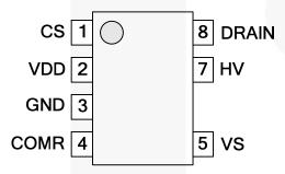
Figure 5. Pin Configuration
