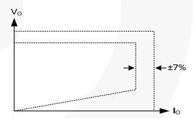
Figure 1. Typical Output V-I Characteristic
