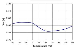
Figure 10. Reference Voltage (V<sub>VR</sub>) vs. Temperature
