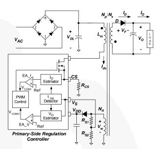
Figure 24. Simplified PSR Flyback Converter Circuit
