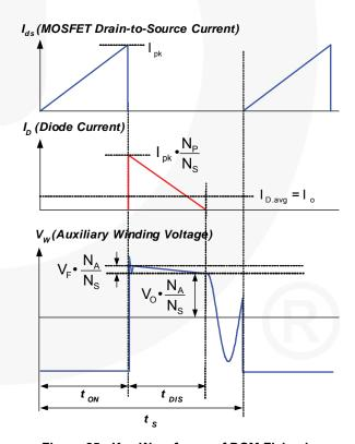
Figure 25. Key Waveforms of DCM Flyback
