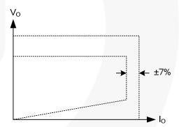
Figure 1. Typical Output V-I Characteristic
