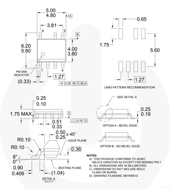
Figure 33. 7-Lead, Small-Outline Integrated Circuit Package (SOIC)
