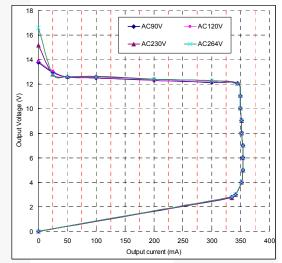
Figure 30. Measured Efficiency and Output Regulation
