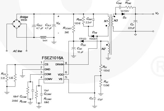
Figure 31. Schematic of Typical Application Circuit
