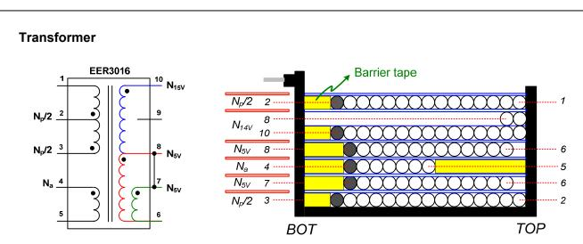
Figure 26. Schematic of Transformer
