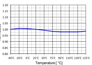
Operating Switching Current (I<sub>OPS</sub>) vs. T<sub>A</sub>
