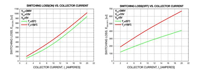
Figure 5. Switching Loss Characteristics
