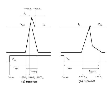
Figure 4. Switching Time Definition
