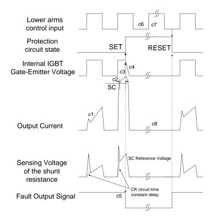
(with the external shunt resistance and CR connection)
