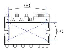
Figure 7. Flatness Measurement Position
