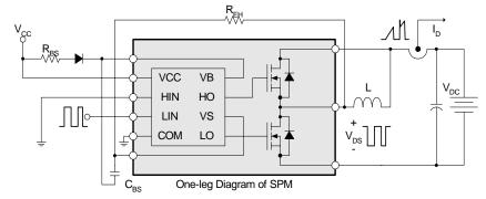
Figure 5. Switching and RBSOA(Single-pulse) Test Circuit (Low-side)
