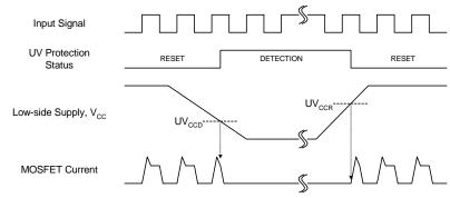
Figure 6. Undervoltage Protection (Low-side)
