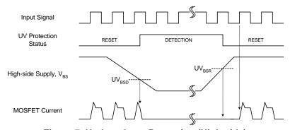
Figure 7. Undervoltage Protection (High-side)
