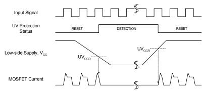
Figure 6. Undervoltage Protection (Low-side)
