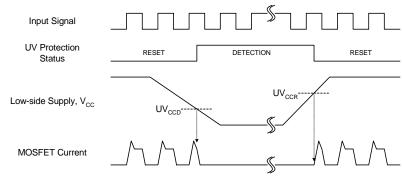
Figure 6. Undervoltage Protection (Low-side)
