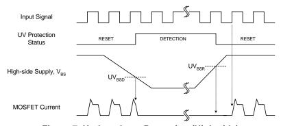
Figure 7. Undervoltage Protection (High-side)
