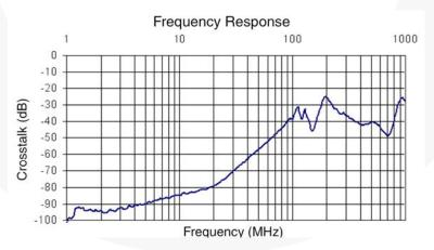
Figure 6. Crosstalk (V<sub>BAIS</sub>=0.5V, V<sub>CC</sub>=3. 0V, SEL<sub>n</sub>=HIGH)
