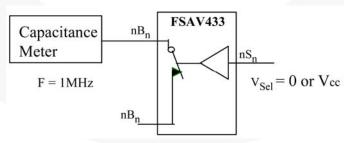
Figure 17. Channel On Capacitance
