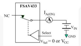
Figure 11. On Leakage
