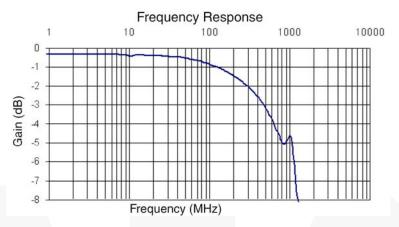
Figure 4. Gain vs. Frequency ( $V_{BAIS}=0.5V$ ,  $V_{CC}=3.6V$ ,  $R_L=50\Omega$ )
