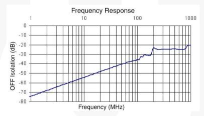
Figure 5. Off Isolation ( $V_{BAIS}=0.5V$ ,  $V_{CC}=3.0V$ ,  $SEL_n=LOW$ )
