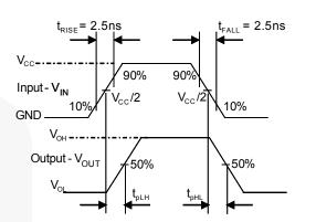
Figure 13. Switch Propagation Delay Waveforms
