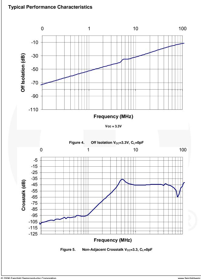
FSA2367 Low  $R_{oN}$  (0.75 $\Omega$ ) Triple-SPDT, Negative-Swing Audio Source Switch
