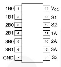
Figure 2. Pin Assignment TSSOP-14 (Top View)
