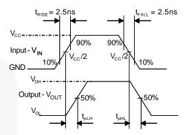
Figure 13. Switch Propagation Delay Waveforms
