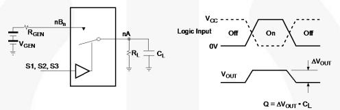
Figure 14. Charge Injection Test (Q=∆V<sub>OUT</sub> \* C<sub>L</sub>)
