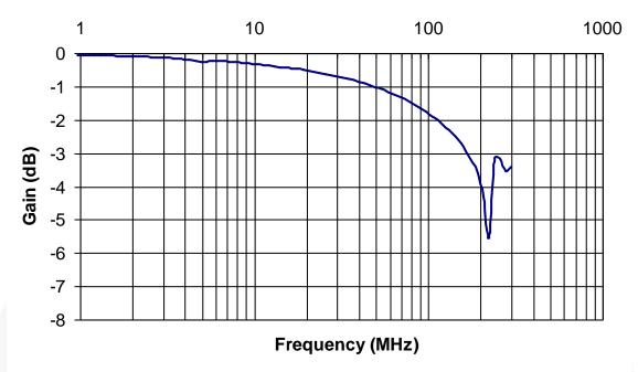
Figure 6. Bandwidth Characterization, Frequency Response at V<sub>CC</sub>=3.3V, C<sub>L</sub>=0pF
