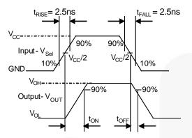
Figure 12. Turn-On / Turn-Off Waveforms
