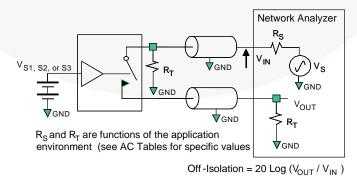
Figure 16. Channel Off Isolation
