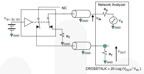
Figure 17. Non-Adjacent Channel-to-Channel Crosstalk
