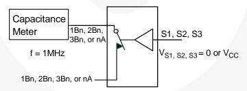
Figure 19. Channel On Capacitance
