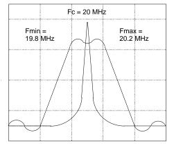
Figure 3. Spectrum Analysis of 19.8 – 20.2 MHz Clock
