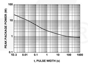
Figure 11. Single-Pulse Maximum Power vs. Time
