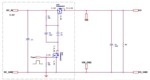
Figure 15. Startup Test Circuit - No Reverse Polarity Protection
