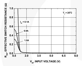
Figure 8. Effective Switch Resistance  $R_{\text{SW}}$  vs. Input Voltage  $V_{\text{IN}}$
