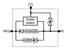
Figure 1. Block Diagram
