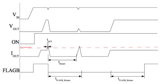
Figure 4. OCP Turn-Off Timing Diagram
