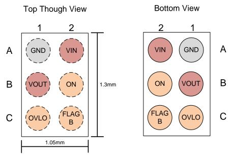
Figure 2. Pin Assignments
