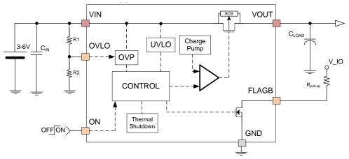
Figure 1. Block Diagram and Typical Application
