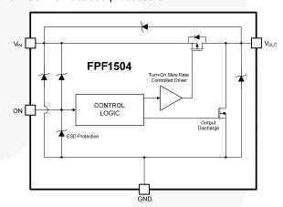
Figure 1. Block Diagram
