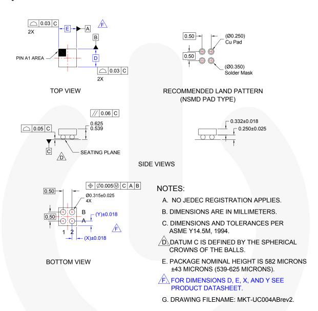
Figure 25. 4-Ball, 1.0 x 1.0mm Wafer-Level Chip Scale (WLCSP) Packaging
