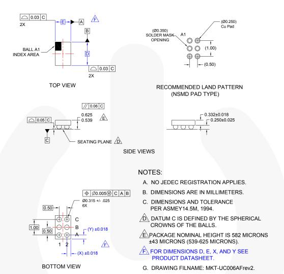
Figure 30. 6 Ball, 1.0 x 1.5 mm Wafer-Level Chip-Scale Packaging (WLCSP)
