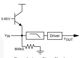
Figure 9. Input Clamp Circuit
