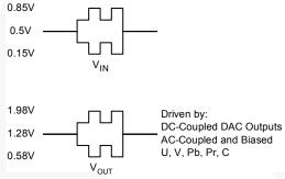
Figure 8. Typical Voltage Levels
