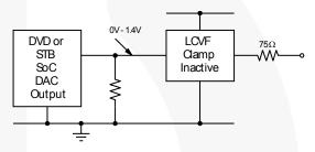
Figure 10. DC-coupled Inputs and Outputs
