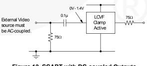
Figure 12. SCART with DC-coupled Outputs
