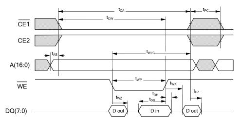
Write Cycle Timing 2 (/CE-Controlled)
