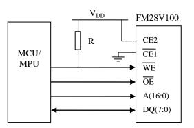
Figure 4. Use of Pullup Resistor on /WE
