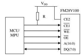
Figure 3. Typical Application using Pullup Resistor on /CE1
