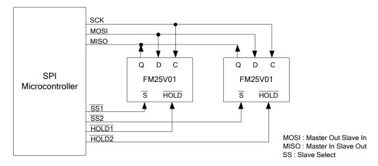
Figure 3. 256Kbit (32KB) System Configuration with SPI port
