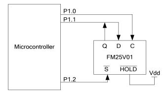
Figure 4. System Configuration without SPI port
