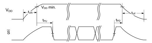
Power Cycle & Sleep Timing  $(T_A = -40^{\circ} \text{ C to} + 85^{\circ} \text{ C}, V_{DD} = 2.0 \text{ V to } 3.6 \text{ V}, \text{ unless otherwise specified})$
