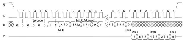
Figure 10. Memory Read with 2-Byte Address
