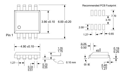
Refer to JEDEC MS-012 for complete dimensions and notes. All dimensions in <u>millimeters</u>.
