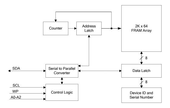
Figure 1. FM24V01 Block Diagram
