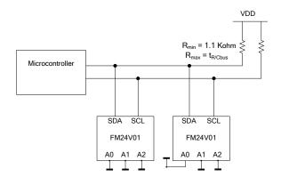
Figure 2. Typical System Configuration
