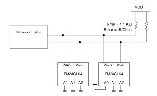
Figure 2. Typical System Configuration
