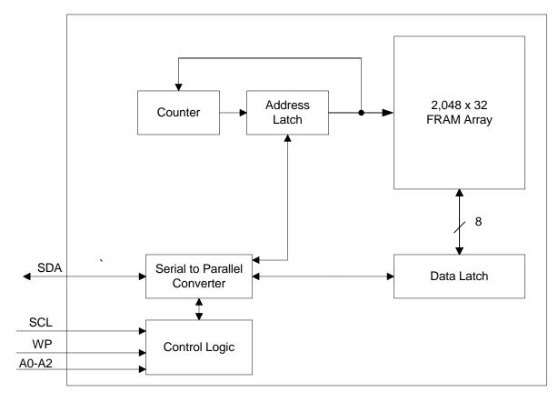
Figure 1. FM24CL64 Block Diagram
