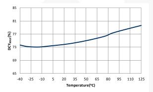
Figure 20. Maximum Duty Cycle (DCY $_{\rm MAX}$ ) vs. Temperature
