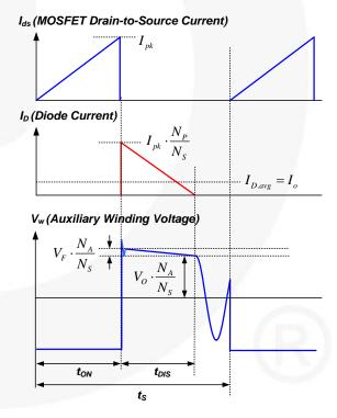
Figure 22. Key Waveforms of DCM Flyback
