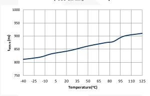
Figure 15. Minimum On Time at No Load (t<sub>MIN-N</sub>) vs. Temperature
