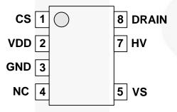
Figure 5. Pin Configuration
