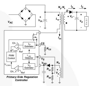
Figure 21. Simplified PSR Flyback Converter Circuit
