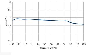
Figure 19. Leakage Current after Startup (I<sub>HV-LC</sub>) vs. Temperature
