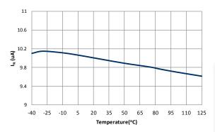
Figure 18. IC Bias Current (Itc) vs. Temperature
