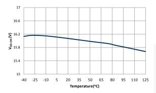
Figure 6. Turn-on Threshold Voltage(V<sub>DD-ON</sub>) vs. Temperature
