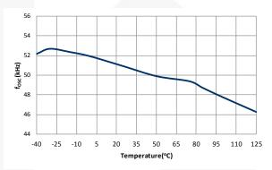
Figure 9. Normal Frequency 1 (fosc) vs. Temperature
