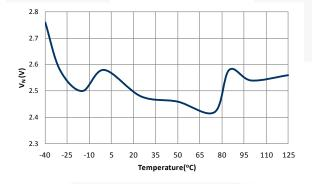
Figure 16. Green Mode Starting Voltage on EA\_V  $(V_N)$  vs. Temperature
