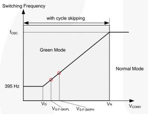
Figure 23. Switching Frequency in Green Mode
