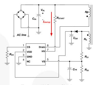
Figure 24. HV Startup Circuit
