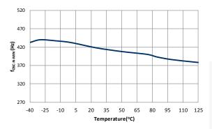
Figure 12. Minimum Frequency at No Load (f<sub>OSC-N-MIN</sub>) vs. Temperature
