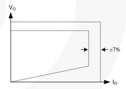
Figure 1. Typical Output V-I Characteristic
