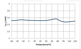
Figure 8. Operating Current (I<sub>DD-OP</sub>) vs. Temperature
