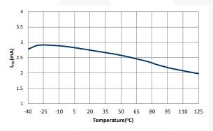
Figure 14. Supply Current Drawn from HV Pin (I<sub>HV</sub>) vs. Temperature
