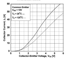
Figure 5. Saturation Voltage vs. Case
