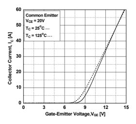
Figure 6. Saturation Voltage vs.  $V_{GE}$
