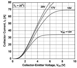
Figure 3. Typical Saturation Voltage Characteristics
