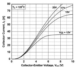
**Figure 4. Transfer Characteristics**
