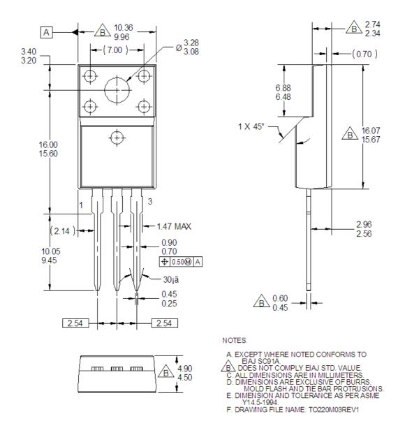
\* Front/Back Side Isolation Voltage: AC 2700V
