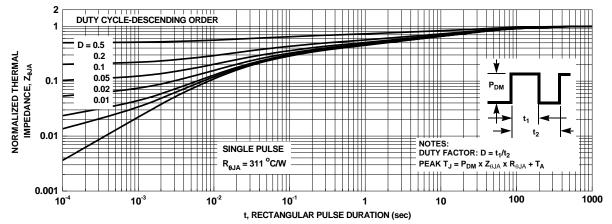
Figure 12. Junction-to-Ambient Transient Thermal Response Curve
