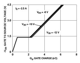
Figure 7. Gate Charge Characteristics
