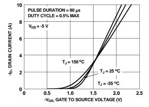
Figure 5. Transfer Characteristics
