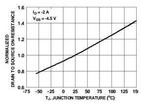
Figure 3. Normalized On-Resistance vs Junction Temperature
