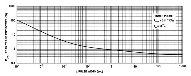
Figure 11. Single Pulse Maximum Power Dissipation
