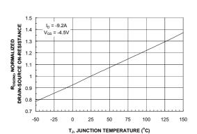
Figure 3. On-Resistance Variation with Temperature.
