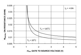
Figure 4. On-Resistance Variation with Gate-to-Source Voltage.
