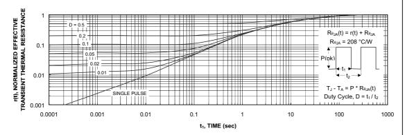
Figure 11. Transient Thermal Response Curve.
