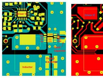
Figure 3.Top/Component (green) View and Bottom (red) PCB View
