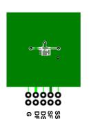
a. 77 °C/W when mounted on a 1 in<sup>2</sup> pad of 2 oz copper
