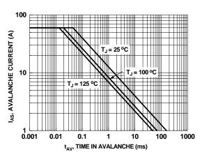
Figure 22. Unclamped Inductive Switching Capability
