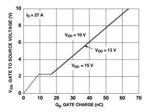
Figure 20. Gate Charge Characteristics
