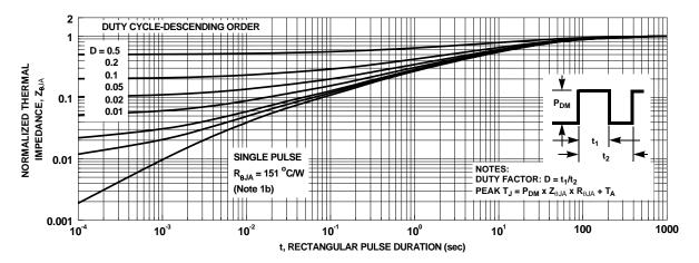
Figure 13. Junction-to-Ambient Transient Thermal Response Curve
