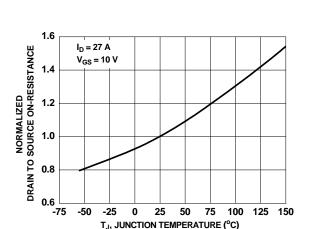
Figure 16. Normalized On-Resistance vs Junction Temperature
