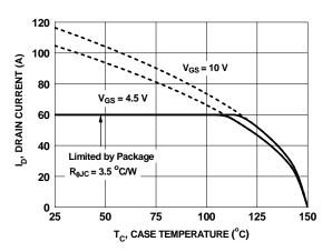
Figure 23. Maximum Continouns Drain Current vs Ambient Temperature
