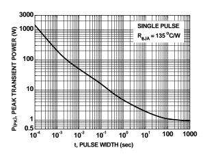
Figure 25. Single Pulse Maximum Power Dissipation
