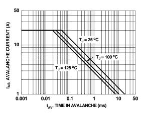
Figure 9. Unclamped Inductive Switching Capability
