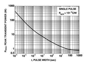
Figure 12. Single Pulse Maximum Power Dissipation
