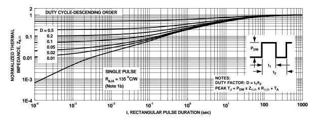
Figure 26. Junction-to-Ambient Transient Thermal Response Curve
