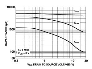
Figure 21. Capacitance vs Drain to Source Voltage
