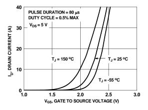
Figure 5. Transfer Characteristics
