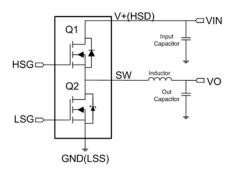
Figure 1.Power Clip in Buck Converter Topology
