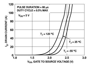
Figure 18. Transfer Characteristics
