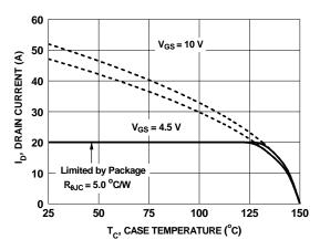
Figure 10. Maximum Continuous Drain Current vs. Ambient Temperature
