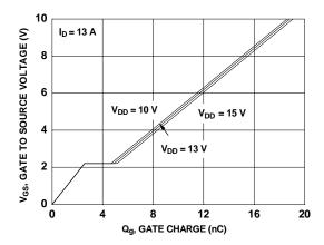
Figure 7. Gate Charge Characteristics
