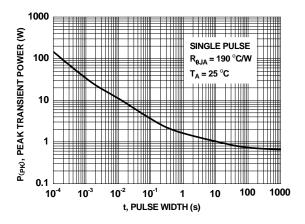
Figure 12. Single Pulse Maximum Power Dissipation
