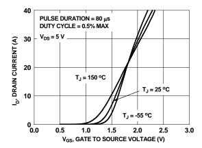
Figure 5. Transfer Characteristics
