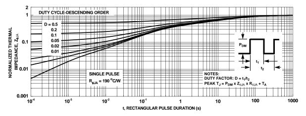
Figure 13. Junction-to-Ambient Transient Thermal Response Curve
