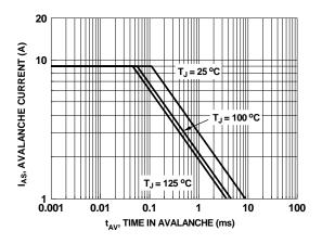
Figure 9. Unclamped Inductive Switching Capability
