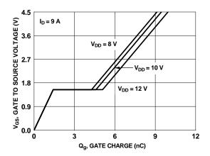
Figure 7. Gate Charge Characteristics
