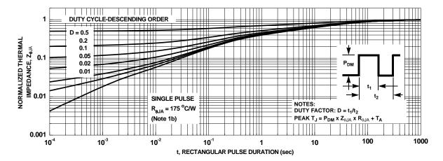
Figure 11. Junction-to-Ambient Transient Thermal Response Curve
