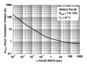
Figure 10. Single Pulse Maximum Power Dissipation
