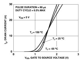
Figure 5. Transfer Characteristics
