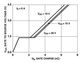
Figure 7. Gate Charge Characteristics
