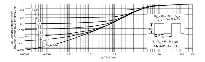
Figure 13. Transient Thermal Response Curve.
