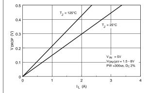
Figure 1.  $V_{DROP}$  Versus  $I_L$  at  $V_{IN} = 5V$ .
