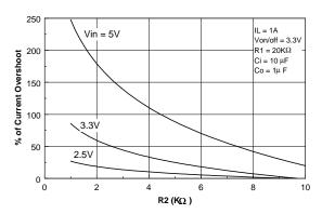
Figure 8. Switching Variation with R2 at Vin = 2.5V and R1 = 20K0hm.
