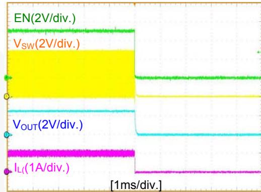
Figure 5. EN Turn off with 1A Load
