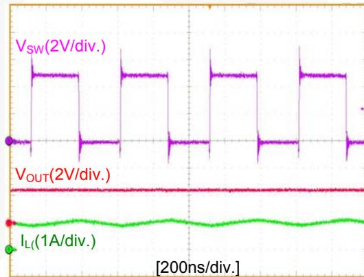
Figure 7. 2MHz Sync Operation with 1A Load
