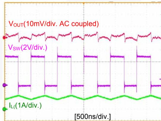
Figure 9. Output Voltage Ripple with 1A Load
