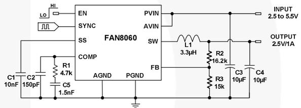
**Figure 15. Recommended Schematic (5V<sub>IN</sub> to 2.5V<sub>O</sub>)**
