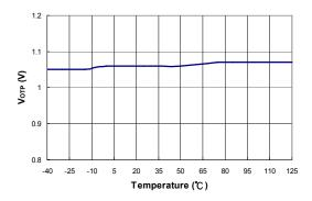
Figure 24. Over-Temperature Protection Threshold Voltage (V<sub>OTP</sub>) vs. Temperature
