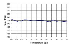
Figure 21. Debounce Time of FB Pin Open-Loop Protection (t<sub>D-OLP</sub>) vs. Temperature
