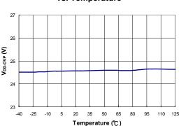
Figure 22.  $V_{DD}$  Over-Voltage Protection ( $V_{DD\text{-}OVP}$ ) vs. Temperature
