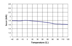
Figure 13. Operation Supply Current (I<sub>DD-OP1</sub>) vs. Temperature
