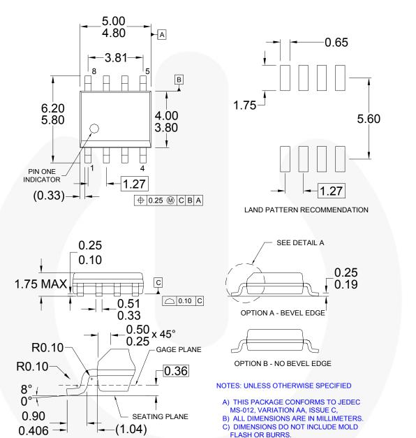
Figure 28. 8-Lead, Small Outline Integrated Circuit (SOIC) Package
