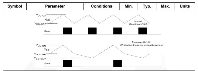
Figure 6. Normal UVLO and Two-Step UVLO Behavior
