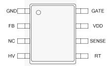
Figure 4. Pin Assignments
