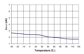
Figure 17. HV Pin Leakage Current After Startup (I<sub>HV-LC</sub>) vs. Temperature
