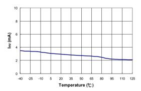
Figure 16. Supply Current Drawn from HV Pin (I<sub>HV</sub>) vs. Temperature
