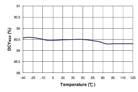
Figure 19. Maximum Duty Cycle (DCY<sub>MAX</sub>) vs. Temperature
