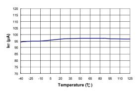
Figure 23. Output Current from RT Pin (I<sub>RT</sub>) vs. Temperature
