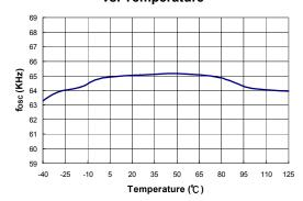
Figure 18. Frequency in Normal Mode (fosc) vs. Temperature
