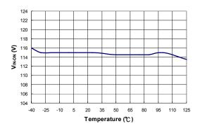
Figure 26. Brown-In (V<sub>IN-ON</sub>) vs. Temperature
