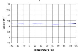
Figure 15. Minimum Operating Voltage (V<sub>DD-OFF</sub>) vs. Temperature
