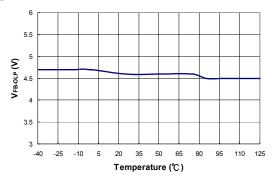
Figure 20. FB Open-Loop Trigger Level (V<sub>FB-OLP</sub>) vs. Temperature
