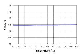
Figure 14. Start Threshold Voltage (V<sub>DD-ON</sub>) vs. Temperature
