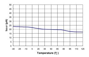
Figure 12. Startup Current (I<sub>DD-ST</sub>) vs. Temperature
