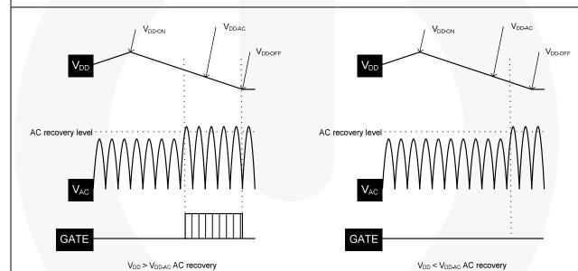
Figure 9. VDD-AC and AC Recovery
