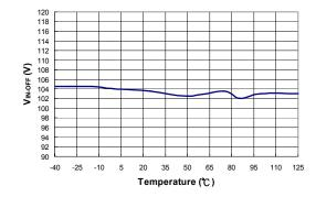
Figure 27. Brownout (V<sub>IN-OFF</sub>) vs. Temperature
