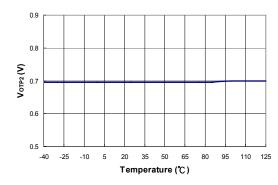
Figure 25. Over-Temperature Protection Threshold Voltage (V<sub>OTP2</sub>) vs. Temperature
